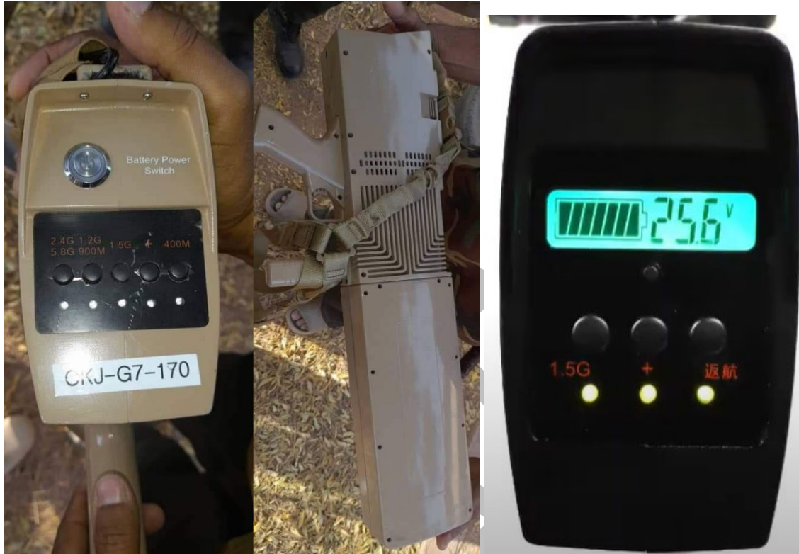
Left: Close-up of the drone jammers, with label marked CKJ-G7-170. 135
